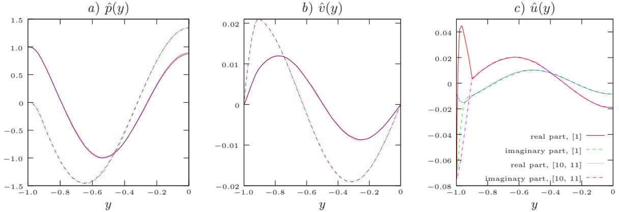
Figure 1: Equivalent of figure 2 of [1]. Mode with  $\omega = -57 - 6.912i \text{ s}^{-1}$ ,  $\alpha = 0.5709 + 5.3453i \text{ m}^{-1}$ .  $\rho_0 = 1.225 \text{ kgm}^{-3}$ ,  $c_0 = 340 \text{ ms}^{-1}$ ,  $h = 1 \text{ m}$ ,  $\delta = 0.1 \text{ m}$ ,  $\bar{U}_0 = 60 \text{ ms}^{-1}$ ,  $U_0(y) = -(y+h)(y+h-2\delta)\bar{U}_0/\delta^2$  for  $y \in [-h, -h+\delta]$ ,  $Z$  is given by (4) with  $d = 0.986$ ,  $b = 1$  and  $R = 2.6 \times 10^{-3}$ .
