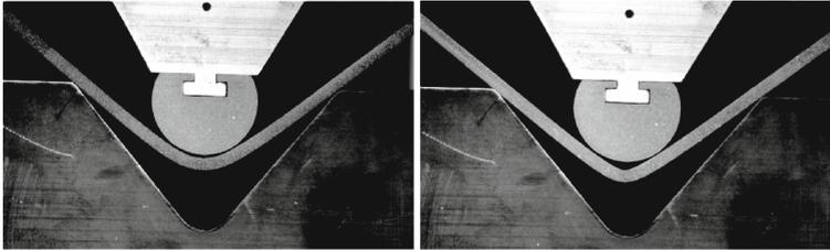
**Fig. 3.** Visual representation of punch-sheet separation. Each photograph shows the same bend conditions and material. Left shows the specimen wrapped around the punch in an ideal scenario. Right shows punch-sheet separation, with a gap appearing underneath the center of the punch. 5 mm thickness, R20 punch.
