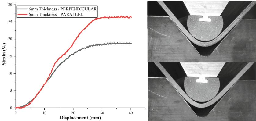
**Fig. 7.** LEFT: 6 mm sheets tested with R25 punch. Specimen presented in red showed punch-sheet separation, while specimens displayed in black did not. UPPER RIGHT: DF27A2 FS2 specimen not displaying punch-sheet separation. LOWER RIGHT: DF27A5 FS1 specimen displaying punch-sheet separation.
