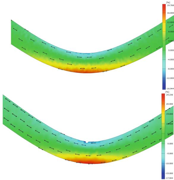
**Fig. 4.** Strain distribution at maximum punch displacement from DIC. 5 mm sheet thickness and R20 punch. TOP: Strain distribution for specimen not displaying punch-sheet separation. BOTTOM: Strain distribution for specimen displaying punch-sheet separation. The missing notch in the center is due to an unresolved section, as opposed to damage or cracking.
