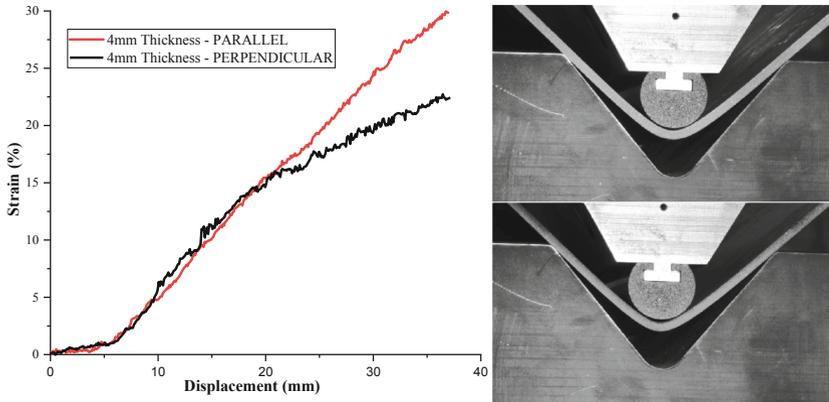
**Fig. 6.** LEFT: 4 mm specimens tested with R15 punch; specimen presented in red showed clear visual punch-sheet separation. UPPER RIGHT: Specimen with the bend line perpendicular to the rolling direction not displaying punch-sheet separation. LOWER RIGHT: Specimen with the bend line parallel to the rolling direction displaying punch-sheet separation.
