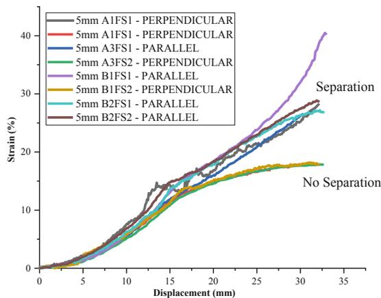
**Fig. 5.** Maximum strain measured on the sheet edge for 5 mm thickness specimens tested with the R20 punch. Specimens that showed separation reached higher strains. Specimens that did not separate averaged at a maximum of 17.8% at maximum punch displacement.
