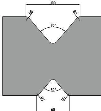
**Fig. 1.** Dimensions of the “Butterfly” V-die configuration. Only results from the larger die (top) are presented here.
