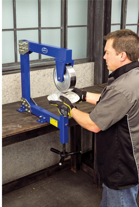
Fig. 1.6 A doubly curved sheet being rolled with an Eastwood English Wheel. Photograph by Nick Capinski.
