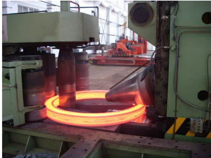
Fig. 1.5 A ring being rolled by a D53K CNC radial axial Ring Rolling Machine. On the left, the ring is pinched between the work roll outside and the mandrell inside. On the right, two horizontal conical rolls prevent vertical growth. Two unpowered guide rolls are also visible on the left, either side of the work roll. As the ring increases in diameter, the left and right sets of rolls are moved apart.
